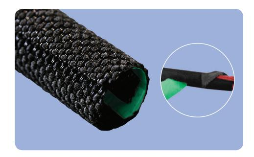
**ROUNDIT® 2000 ST** is a self-closing oversleeve designed to provide mechanical protection. ROUNDIT 2000 ST is made out of a woven substrate of monofilament and multifilament polyester yarns equipped with an adhesive tape. This unique design gives the adhesive tape the double advantage of holding the sleeve in place on the application and being a secure closing system.
